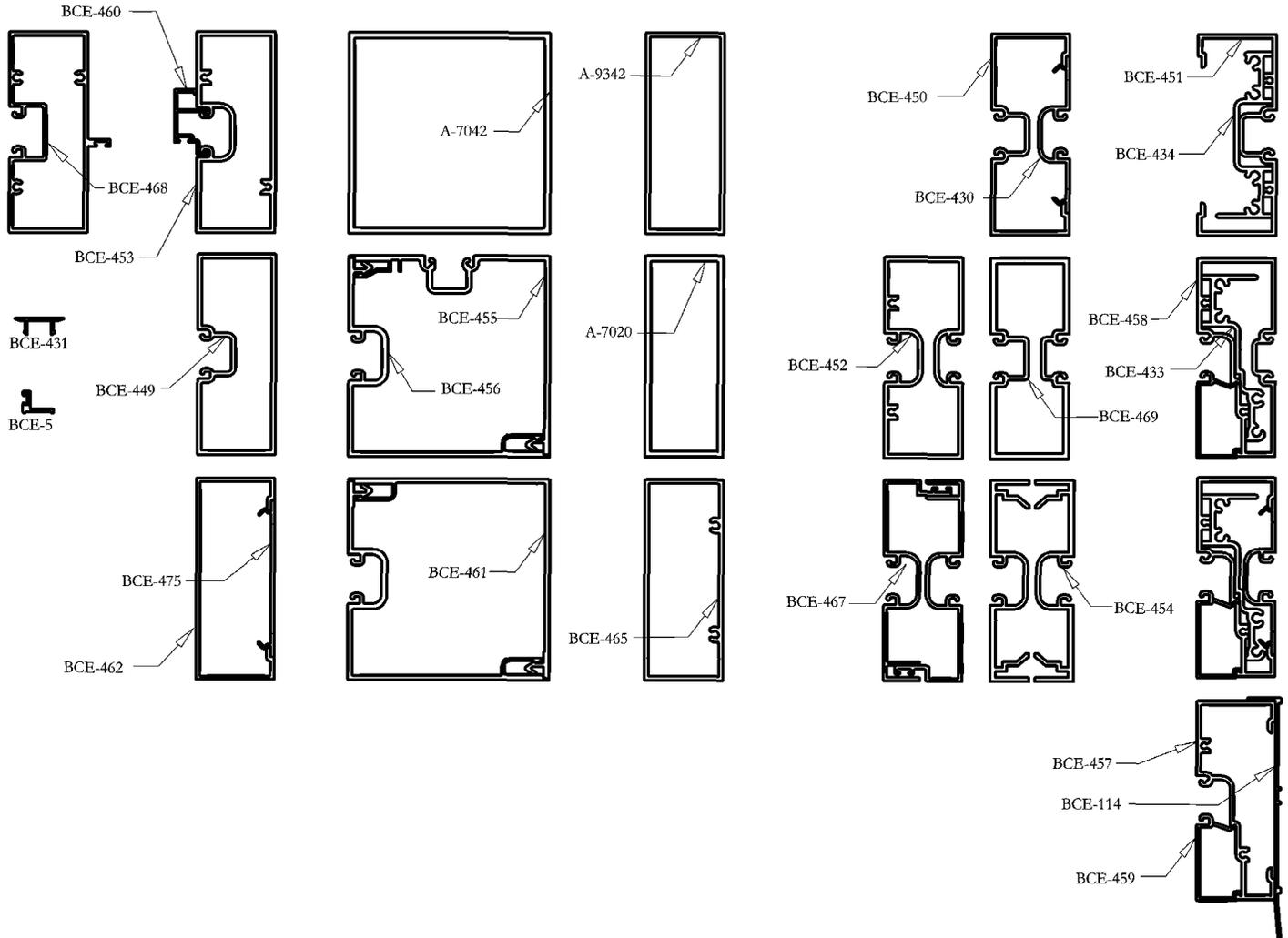
THIS SYSTEM IS DESIGNED TO BE ASSEMBLED WITH #8 SCREWS EXCEPT WHERE NOTED
